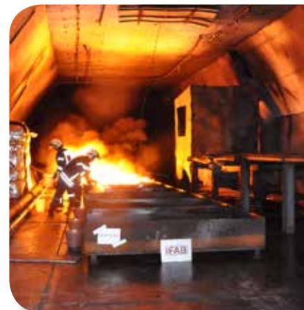
Tunnel Mont Blanc fire tests with different fixed fire fighting systems
