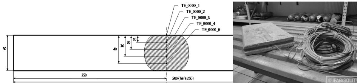
**Figure 1:** Sketch and photograph of a concrete specimen and assembled material thermocouples
