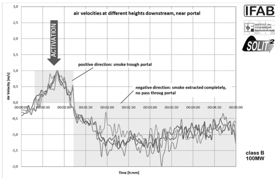
**Figure 6:** Air velocities near the downstream tunnel portal during a 100 MW class B fire test
