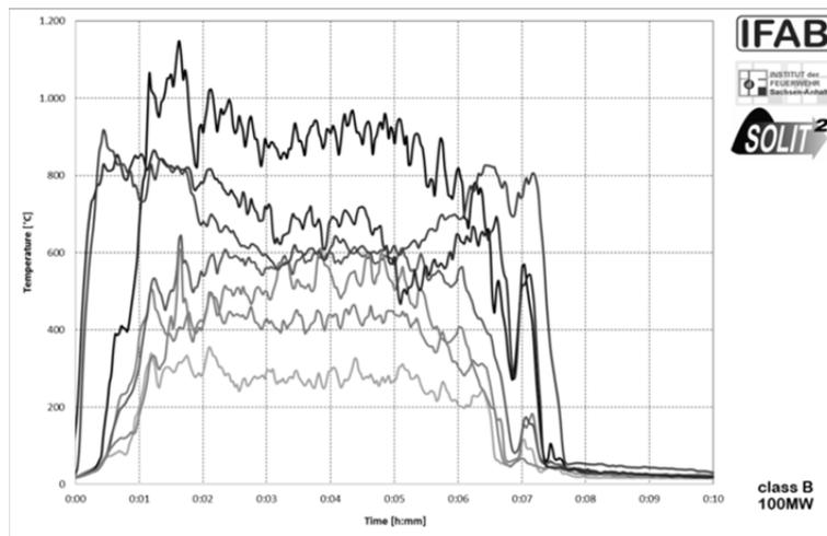
**Figure 4:** Temperatures near the fire zone at different heights during a 100 MW class B fire test
